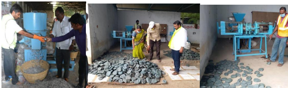
Figure 2.2: Granule machine or also called polythene chips maker machine
